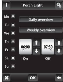
Having entered the weekly program function for the required 'switching' location/circuit you arrive at this screen. Select the day and times and then press OK. Repeat the process for additional programs.
