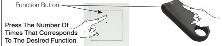
Each time the transmitter button is pressed the LED on the receiver will also flash to confirm the signal has been received.
