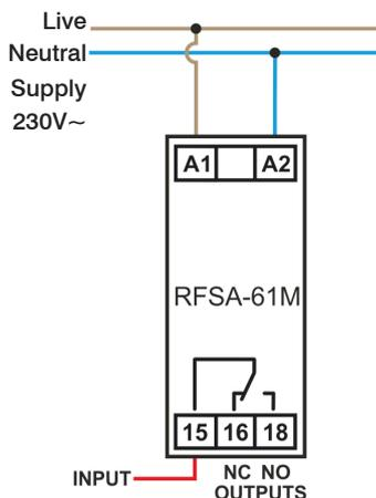
16A switching receiver with option of normally closed and/or normally open contacts.
