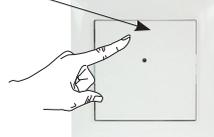
**Press The Transmitter Button Once To Remove.**
