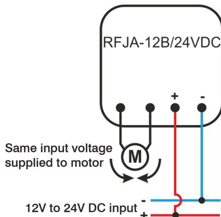
Ensure the correct type of receiver is selected to prevent damage to the motor or receiver
