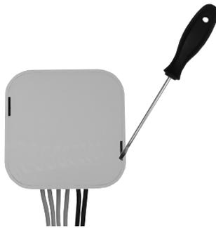
1. Remove rear cover to reveal battery compartment
