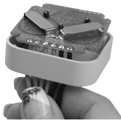
2. Carefully feed cables through housing
