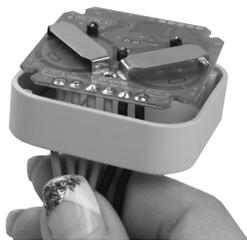
2. Carefully feed cables through housing
