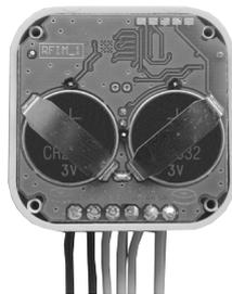
4. Carefully slide PCB back in to the housing
