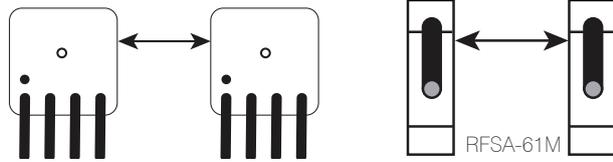
2. Box receivers, stagger each one. So one towards the back and the next towards the front. This helps the signal to reach the required receiver if controlled from the side.
