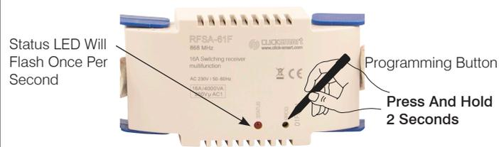
The program button may be recessed in to the body, this is standard. A small implement e.g. stylus can be used to press and hold the button.
