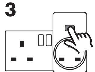
While the green light is flashing press the "Status/Prog" button again. The light should now flash red for 5 seconds then no light will appear. This indicates the unit is in "Learning Mode".
