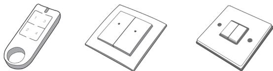
Still while no indicator lights are illuminated on the repeater; use the control that is paired with the receivers you wish to assign to the repeater. Press a button/switch on the control to turn the receiver on. The repeater status light should flash green once to indicate the pairing has been made.
