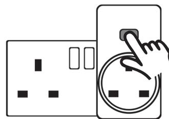
Once you have successfully paired the devices, press the "STATUS/PROG" button to switch to resume normal operation. The green indicator will be constantly illuminated.
