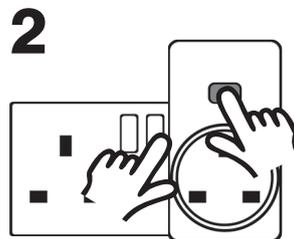
While holding the "Status/Prog" button, switch on the socket. Continue holding the "Status/Prog" button until the red indicator light shows. Release the button. The indicator light will flash green.
