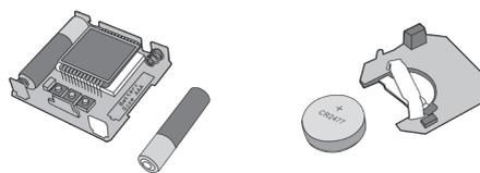
Still while no indicator lights are illuminated on the repeater; insert the battery/batteries into the product. The repeater status light should flash green to indicate the pairing has been made.
